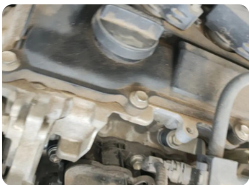
Eng. Valve Cover: Oil leakage present
