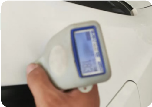
LH C-Pillar Outer: Paint repair present
