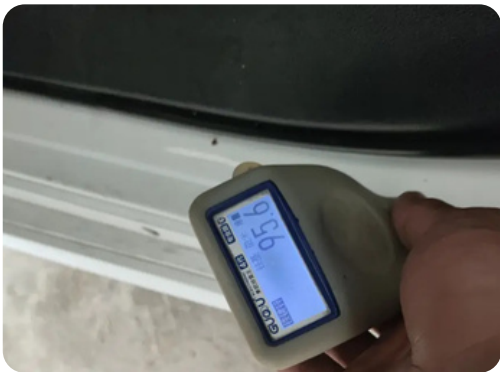
LR Quarter Panel: Paintwork and body repair present ≥20cm
