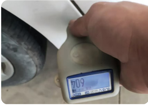
RR Quarter Panel: Paintwork and body repair present \geq 20\text{cm}
