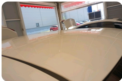
Roof Panel: Depression, 200mm*300mm
